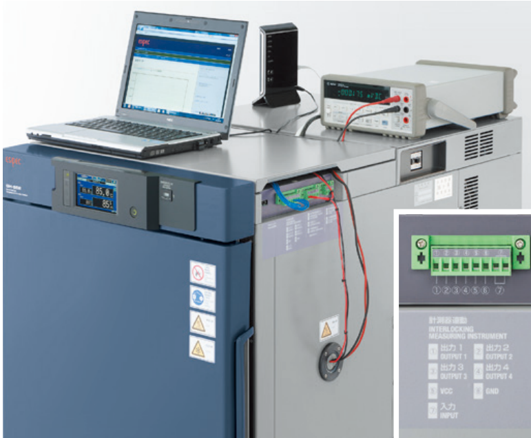
Instrumentation interlock terminals
